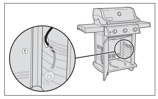
Maximum LPG cylinder capacity OUTSIDE cabinet is 13 kg.
